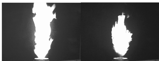
Fig. 13 Images of forced 45/50 deg flame. Left image: Flame near peak heat release. Right image: Flame near minimum heat release.
